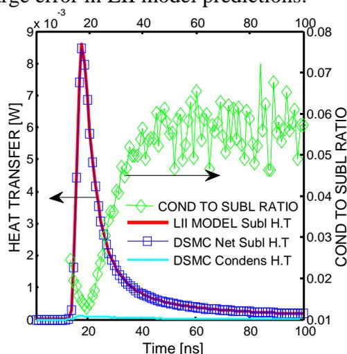
Fig. 2: Nanoparticle cooling decay determined using transient DSMC
