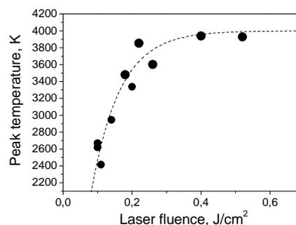
Fig. 2. The dependence of peak temperature of laser heated Mo nanoparticles on laser fluence.
