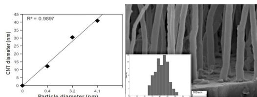
Fig. 4. Linear correlation between the particle size in situ detected by LII and the ex situ measured carbon nanotube (CNT) diameter. There is a direct relationship between the particle formed in the gas phase and the resulting nanotubes. These results present a first step toward the direct control of the CNT structure (i.e. diameter and chirality) during the growth process.
