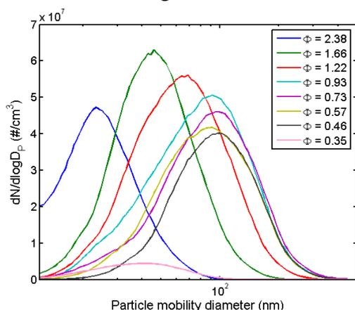
**Figure 1.** SMPS data presenting the particle size distribution for different equivalence ratios ( $\Phi$ ).
