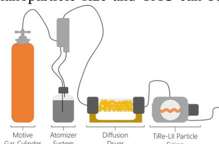
Fig. 1. Schematic of the experimental apparatus.
