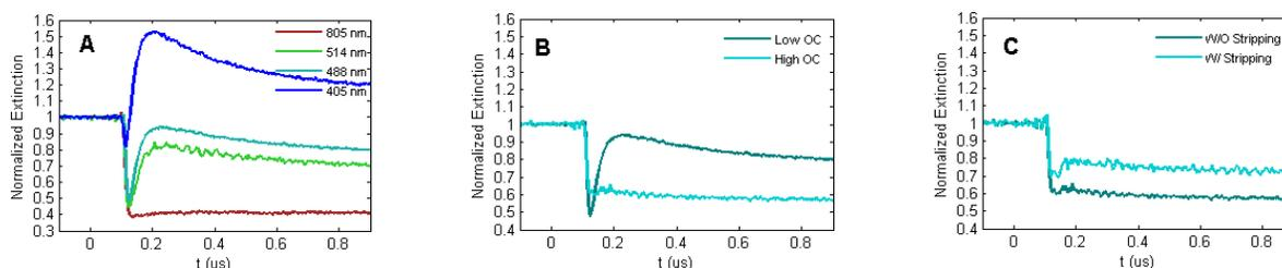
(A) Time-resolved attenuation profiles at four different CW wavelengths for untreated soot with low organic content; (B) Extinction profiles of soot particles with high and low organic carbon levels at 488 nm; (C) Extinction profiles of untreated and stripped organic-rich particles at 488 nm. The IR laser fluence used for all three figures is  $5.45 \text{ mJ/mm}^2$ .
