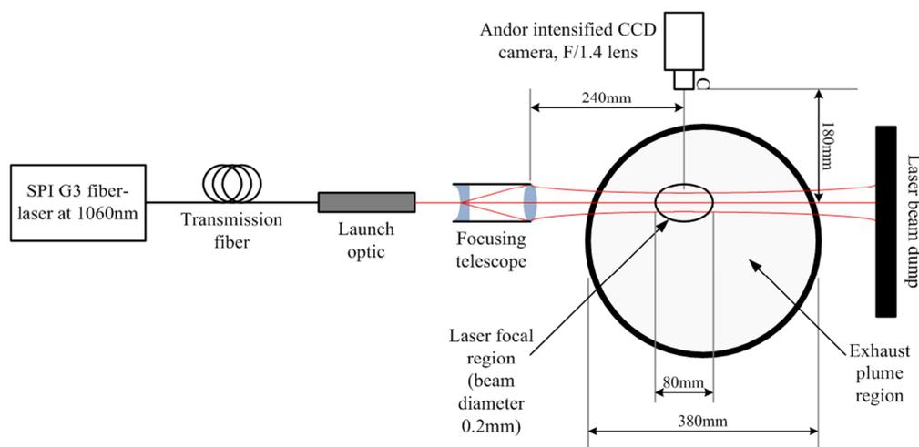
Fig. 1. LII arrangement for experiments on a modified helicopter engine
