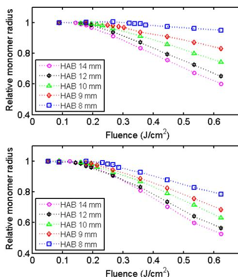
Fig 2. Inferred relative monomer radius from ELS as function of laser fluence at 1064 nm for two flames,  $\Phi = 2.1$  (top graph) and 2.3.
