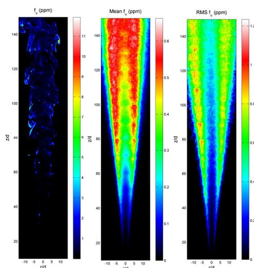
Fig. 1. Stacked LII planar images of instantaneous  $f_v$ , mean  $f_v$  (1000 images) and RMS of  $f_v$  in a turbulent jet flame fueled by prevaporized JP-8 surrogate
