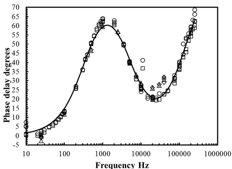
Fig. 1: Measured phase delay of MLII signals with respect to laser excitation source. Open squares, and open circles phase from 445 and 750 nm channels, respectively using 7265 lock-in amplifier. Open triangle, and open diamond phase from 445 and 750 nm channels, respectively using Femto lock-in amplifier. Curve least-mean-squares fit of data using developed theory.
