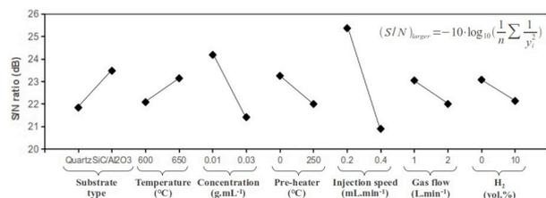
Fig. 3. Analysis of Taguchi robust design method introduced for multifactor process optimization<sup>3</sup>. A set of experiments was designed to investigate the most influential CVD parameters in the cluster size. Seven control factors with two levels were examined, leading to eight experiments organized in a L8 Taguchi matrix design.
