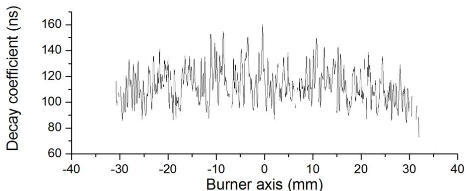
Fig. 1. Exponential decay coefficient across horizontal line at approximately 12 mm height above McKenna burner (equivalence ratio = 2.1, 30 images averaged before calculation of decay coefficient)
