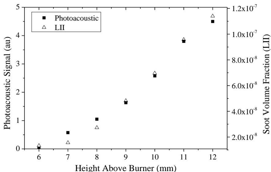
Fig. 1. Comparison of profile obtained from photoacoustic detection with 1064nm LII calibrated to soot volume fraction. These results were taken in a 2.1 equivalence ratio  $\text{C}_2\text{H}_4/\text{Air}$  premixed flame
