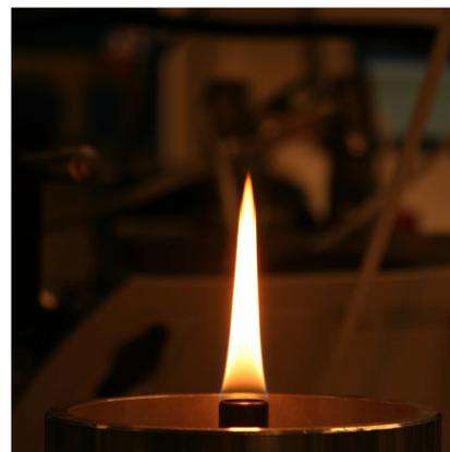
Fig. 2 The ethylene diffusion flame used in this study. Measurements were made at 42 mm height above the burner nozzle.
