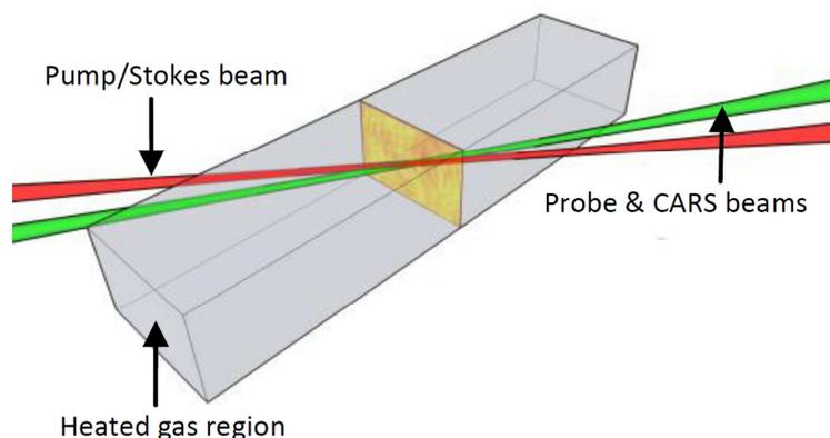
Fig. 1 A sketch of the measurement point, showing the crossing of the heating 1064-nm LII laser beam and the CARS laser beams. The gray box represents the heating laser with a top-hat profile and the CARS beams are indicated by arrows.
