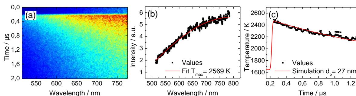
Fig. 1 (a) LII spectral decay. The maximum heat up temperature is fitted via Planck's Law (b). The resulting temperature decay curve is shown in (c). *Squares*: Temperature decay fitted with Planck's law for each time step. *Solid line*: Simulation of the temperature variation based on our heat transfer model.
