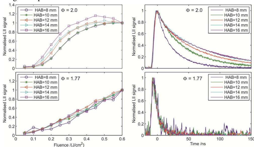
Fig. 1. Fluence curves and time-resolved LII signals (laser fluence  $0.2 \text{ J/cm}^2$ ) for a moderately sooting flame (top) and a flame at the sooting threshold (bottom).
