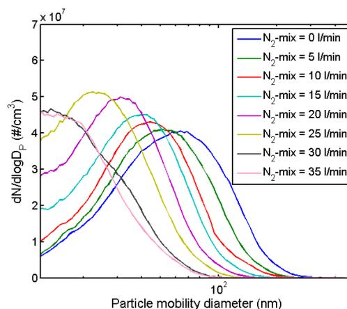
**Figure 2.** SMPS data presenting the particle size distribution as different N<sub>2</sub> mixing gas flows are introduced into the fuel flow.
