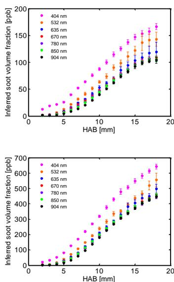
Fig. 1. Inferred soot volume fraction as function of height above burner (HAB) for various laser wavelengths for two flames,  $\Phi = 2.1$  (top graph) and 2.3. Evaluated with  $m = 1.56 - 0.46i^4$
