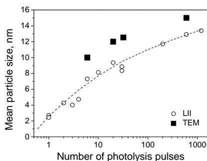
Fig. 1. The mean particle sizes measured by LII and TEM versus number of Kr-F laser pulses.
