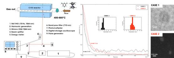
Fig. 2. LII diagnostic in a chemical vapor deposition reactor and comparisons between time-resolved microscopy.
