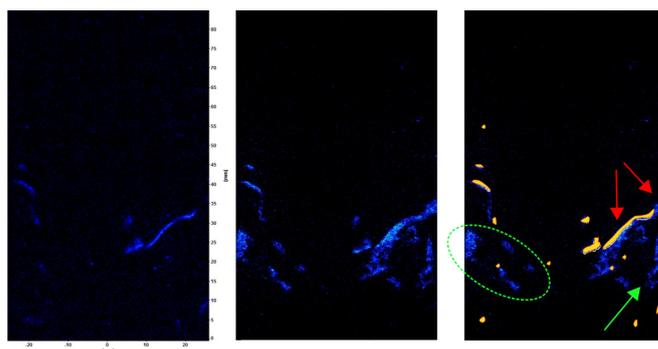
Fig. 1. Left image shows soot distribution (IR excitation), center plot is LIF/LII (UV excitation), right plot visualizes an overlay of the LII contour on the LIF/LII image. Separated PAH clouds are labeled green, transitioning ones into soot red.
