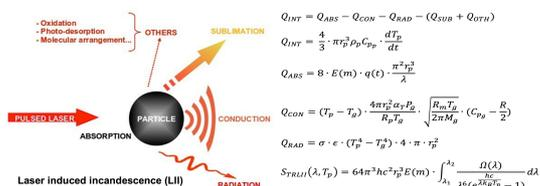
Fig. 1. LII theory and model, in which  $(Q_{SUB} + Q_{OTH})$  sum can be neglected at low laser energy density ( $< 0.6 \text{ J} \cdot \text{cm}^{-2}$ )<sup>1,2</sup>.
