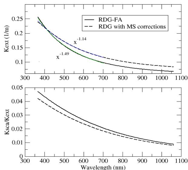
Fig. 1 Impact of aggregate internal multiple scattering on the evaluation of the extinction spectra.
