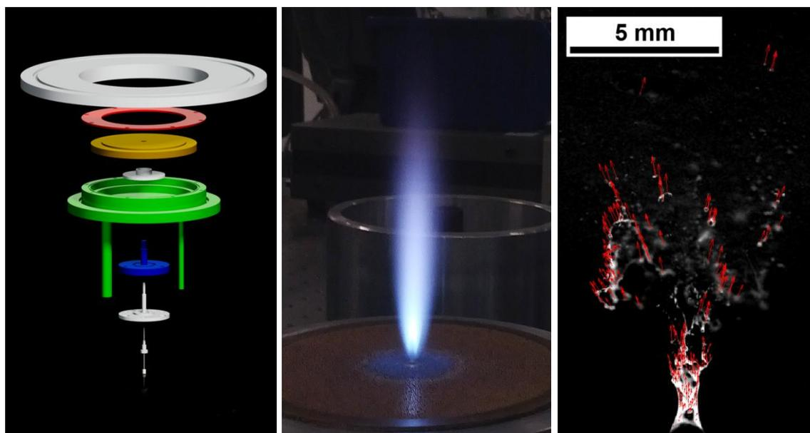
Fig. 1: Left: Assembly drawing of the nozzle of the spray burner, center: Ethanol spray flame, right: Particle tracking velocimetry to determine droplet velocity.
