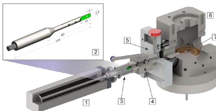
Fig. 1. High-pressure burner with attached TEM-sampler.
