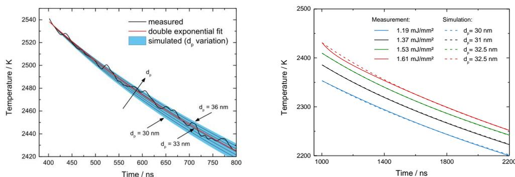
Figure 1. Measured and simulated temperature variation after laser heat-up for various particle diameters  $d_p$  (left); Comparison of measured (double exponential fit, solid lines) and simulated (dashed lines) signal traces for various laser fluences (right).
